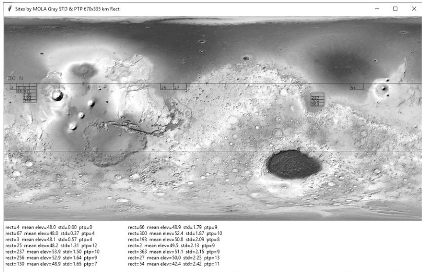
Figure 7-13: Final display with high-graded rectangles and summary statistics sorted by standard deviation
