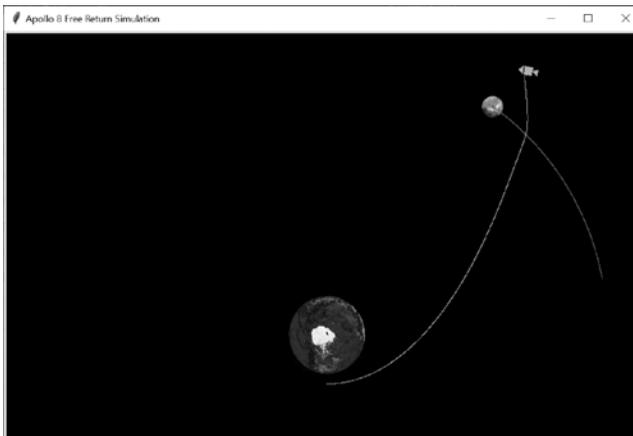
Figure 6-15: The gravitational slingshot maneuver achieved with  $V_{o\_X} = 520$
