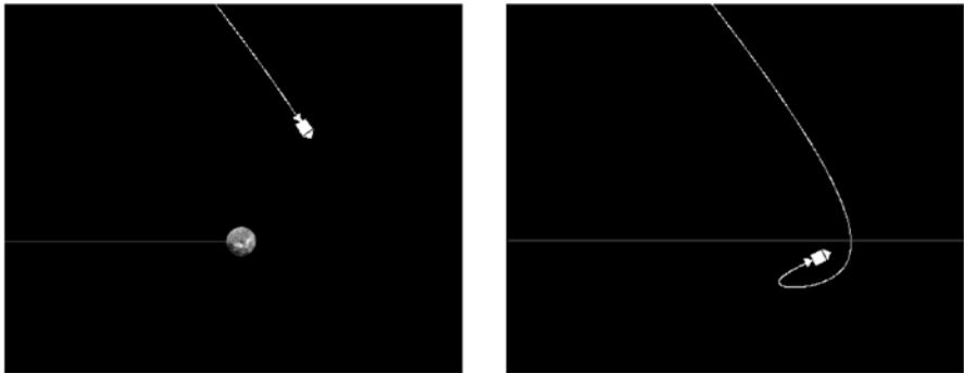
Figure 6-19: The moon and CSM cross orbits, and the moon slows and turns the CSM.
