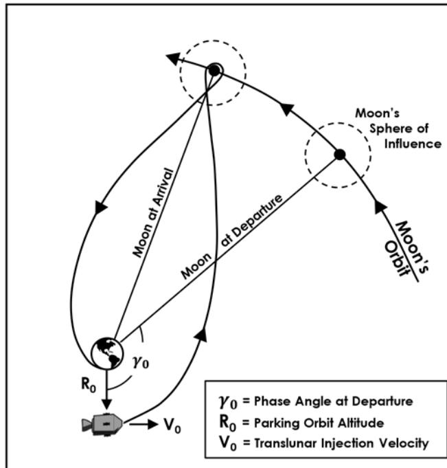
Figure 6-3: The free return trajectory (not to scale)
