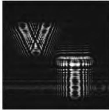
Figure 4.12 Sine-FZP hologram of two letters "V" and "T" located at different depths. Reprinted from T.-C. Poon et al., Optical Engineering 34, 1338 (1995), with permission. © SPIE.
