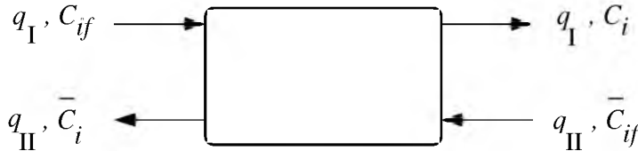
Countercurrent flow of two streams
