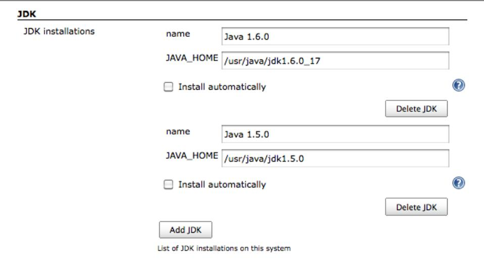
The screenshot shows the 'JDK' configuration page in Jenkins. It features a section titled 'JDK installations' with two entries. Each entry consists of a 'name' field (e.g., 'Java 1.6.0'), a 'JAVA\_HOME' field (e.g., '/usr/java/jdk1.6.0\_17'), and an unchecked 'Install automatically' checkbox. A 'Delete JDK' button is located to the right of each entry. At the bottom of the section, there is an 'Add JDK' button and a link that says 'List of JDK installations on this system'.
