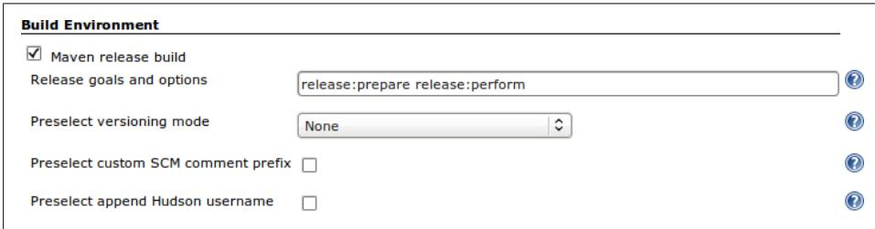
The screenshot shows the 'Build Environment' configuration section. It includes a checked checkbox for 'Maven release build'. Below it, the 'Release goals and options' field contains the text 'release:prepare release:perform'. There are also dropdown menus for 'Preselect versioning mode' (set to 'None') and checkboxes for 'Preselect custom SCM comment prefix' and 'Preselect append Hudson username', both of which are currently unchecked. Each field has a help icon to its right.
