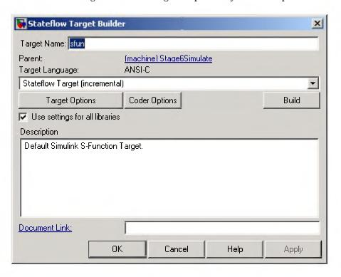
**Note** This dialog box is used to configure Stateflow for building targets. A target is a program that executes a Stateflow chart or a Simulink model that contains a Stateflow chart. Stateflow builds a simulation target (sfun) that lets you simulate your Stateflow application in Simulink. For more information, see "Building Targets" in the online Stateflow User's Guide documentation.
