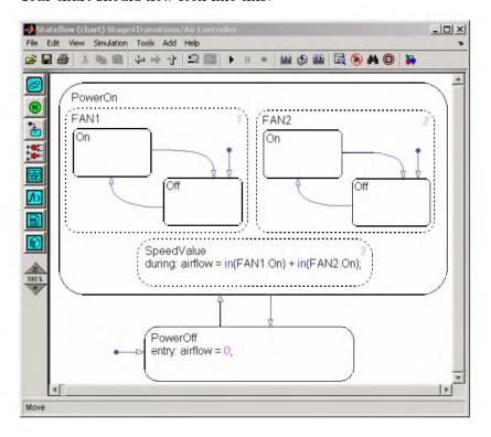
**Tip** The location of the tail of a default transition determines the state it activates. Therefore, you must make sure that your default transition fits completely inside the parent of the state that it activates. In the Air Controller chart pictured above, notice that the default transition for FAN1.Off correctly resides inside the parent state, FAN1. Now consider this chart:
