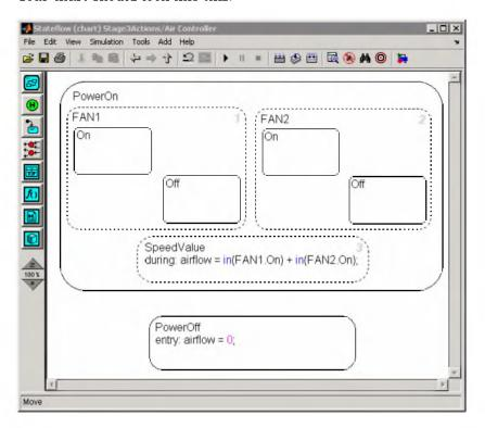
The Boolean expression in (FAN1.0n) is true — and its value equals 1 — if the On state of FAN1 is active. If FAN1 is not on — that is, its Off state is active or power is off — then in (FAN1.On) equals 0. Similarly, the value of in (FAN2.On) represents whether FAN2 is on or off. Therefore, the sum of these Boolean expressions indicates whether 0, 1, or 2 fans are operating during each time step.
