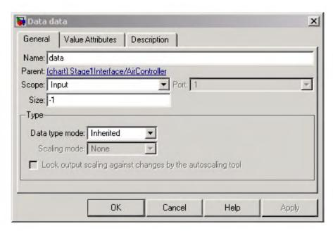
The default values that appear are based on the scope — in this case, a data input.
