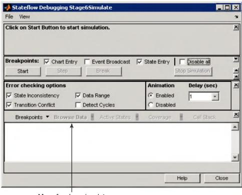
Menu for observing data when simulation pauses at a breakpoint
