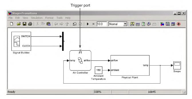
When you define one or more input events for a chart, Stateflow adds a single trigger port to the block. External Simulink blocks can trigger the input events via a signal or vector of signals connected to the trigger port.
