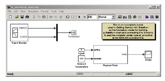
The model is incomplete because it doesn't include the Stateflow chart that you will build as you work through the exercises in this guide. Instead, the model contains several nonfunctional blocks: the Terminator, Inport, and Annotation blocks, as shown:
