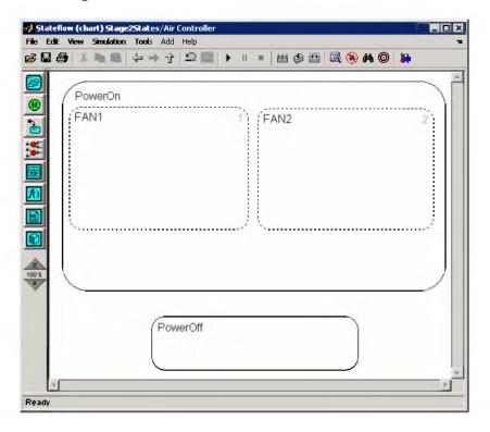
**Note** Your chart may not show the same execution order for parallel substates FAN1 and FAN2. The reason is that, by default, Stateflow orders parallel states based on where they are located in the state diagram. Priority goes from top to bottom and then left to right. If FAN2 is higher in position than FAN1 in your diagram, FAN2 moves to the top of the order. You will fine-tune order of activation in a later exercise, "Setting Explicit Ordering of Parallel States" on page 4-14.
