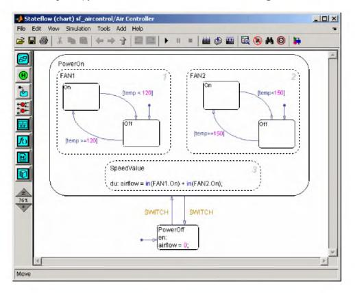
As you can see from the title bar, the Stateflow chart is called Air Controller and is part of a Simulink model called sf\_aircontrol. When you build this chart, you will learn how to work with the following elements of state-transition charts:
