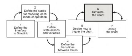
You have entered phase 6 of a basic workflow for building a Stateflow chart: *simulating the chart*. By the time you reach this phase, you have finished building your chart and integrating it with the Simulink model. Now it is time to test the chart by simulating its run-time behavior. During simulation, you can *animate* Stateflow charts to highlight states and transitions as they execute. This chapter guides you through the tasks required for simulating the chart with animation.
