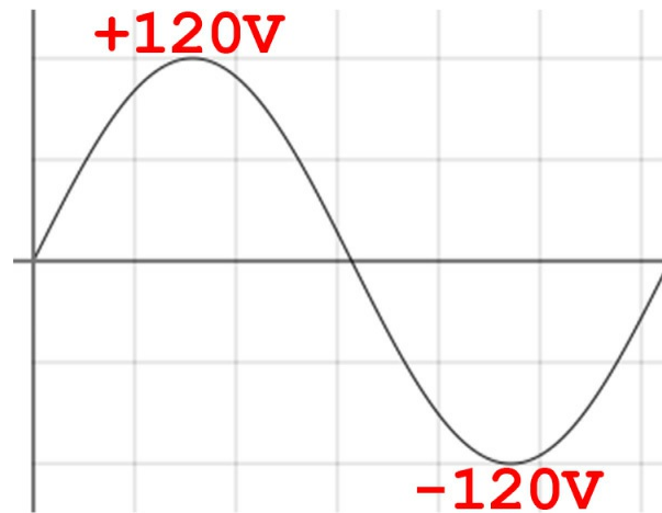
Figure 12.1 Alternating current (AC)
