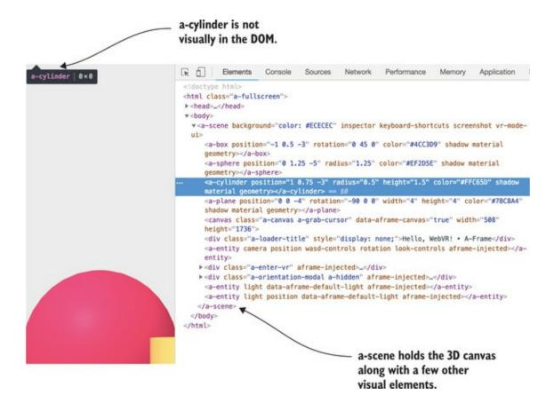
That's because these elements that represent objects in the <a-scene> element aren't actually used visually. A-Frame is using HTML elements as nonvisual data models to be created in 3D. This is interesting, isn't it? On one hand, we have the <a-scene> component handling the incredible complexity of a full 3D scene and also allowing it to work in a variety of VR settings and hardware.
