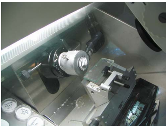
Fig. 14.2 Cryo-microtome chamber with a sample embedded in tissue-freezing media
