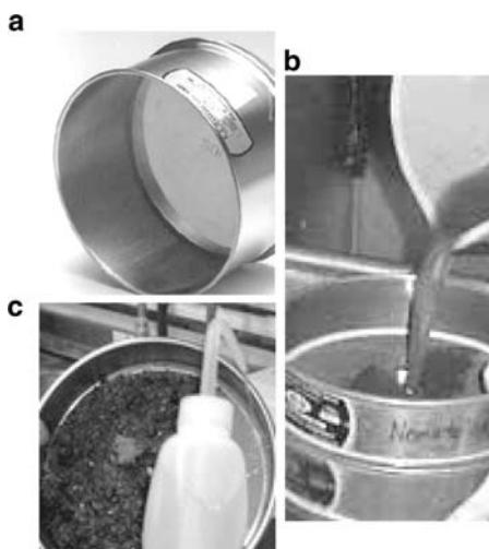
Fig. 10.4 Steps in the wet-sieving technique: (a) metallic sieve, (b) decanting through a sieve series, (c) removal of debris
