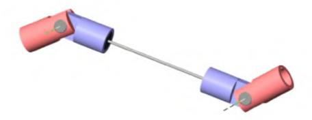
Massless Connector Between Revolute and Revolute Joints
