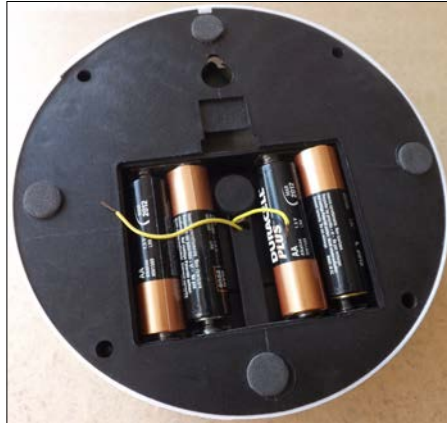
4x AA batteries provide a power source to drive the wheels
