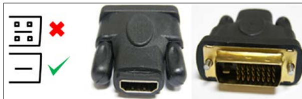
HDMI to DVI connection (DVI-D adaptor)
