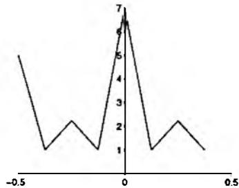
Let us do a slightly more realistic example. We simulate some data recorded at a sampling frequency of 1 kHz, corresponding to a time step  $dt = 1/1000$  of a second. The Nyquist frequency is, therefore, 500 Hz. Suppose there is a 100 Hz sinusoid contaminated by noise. We simulate the data, calculate the FFT, and plot the results as follows:
