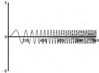
The frequency content of this signal as a function of time can be calculated using the `specgram` function. This function uses the Short Time Fourier Transform (STFT) technique. The STFT chops up the signal into a series of short segments and calculates the FFT of each segment. Each FFT becomes the estimate of the frequency content at that time. For our example we can get a quick display by typing:
