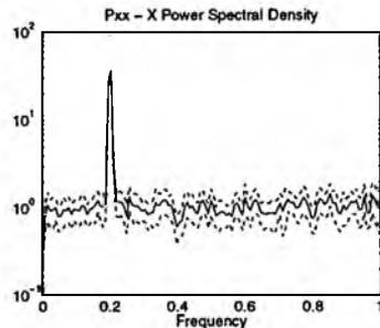
The frequency scale is normalised to the Nyquist frequency. The middle line is the PSD estimate and the two dashed lines are the 95% confidence intervals. Typing `help spectrum` reveals that there are many parameters that you can adjust when calculating the power spectrum. MATLAB’s `spectrum` function uses the Welch method of PSD estimation,<sup>6</sup> which divides a long signal into a number of smaller blocks, calculates
