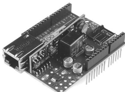
Arduino Ethernet Shield
